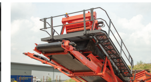
Three sided walkway around main conveyor
