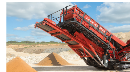
Three sided walkway around main conveyor
